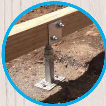
\*Note: The product has a supplied lowest height of approx 175mm. In order to achieve 160mm, the bottom 15-20mm of the threaded rod needs to be cut off.
